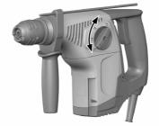
Set the function selector switch to the "Chiseling" position T.
