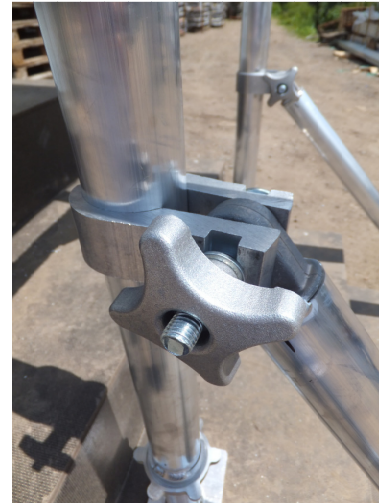
3. POSITION PODIUM, ADJUST LEGS TO LEVEL UNIT AND FIX STABILISERS. TIGHTEN WING NUTS FINGER TIGHT.
