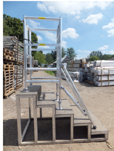
3. POSITION PODIUM, ADJUST LEGS TO LEVEL UNIT AND FIX STABILISERS. TIGHTEN WING NUTS FINGER TIGHT.
