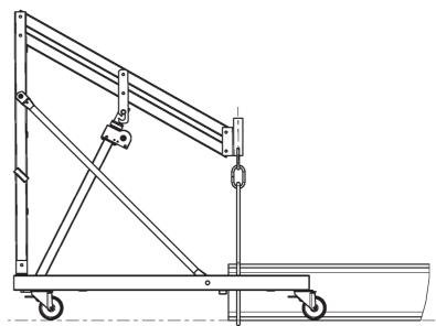
heading fork. This height depends on whether the heading fork is directly inserted into the mounting of the lifting jack or whether the adapter (order no. 12374) is used for a total lifting height of 3.0 m (see below). The lifted carrier is to be placed down on an appropriate load-bearing support (e.g. scaffold jacks).
