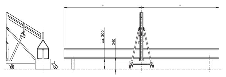
Once the heading fork and adapter, if required, are installed, the carrier (load) is to be lifted again in the centre of gravity. Borings in the plate of the heading fork enable additional mounting of the carrier. It is recommended during the lift to always track the support to provide an additional safety device against tilting and falling. The lifting jack must only be moved in its longitudinal direction with a lifted load!
